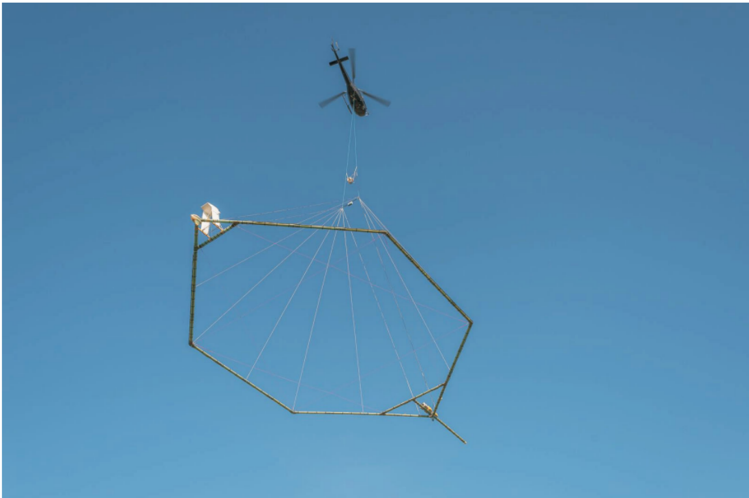
Figure 4: SkyTEM 312 Fast system.
